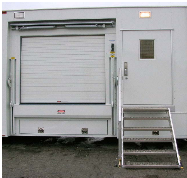
Figure 18: Stair Assembly (standard)
